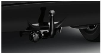
The detachable towing hitch gives you ideal capacity to tow a trailer. It is designed for the Toyota Yaris and has a tough anti-corrosion surface treatment
