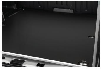
Anti-slip floor protection in Polypropylene material.
